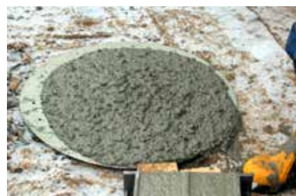
Good workability T-concrete: slump flow > 550 mm
