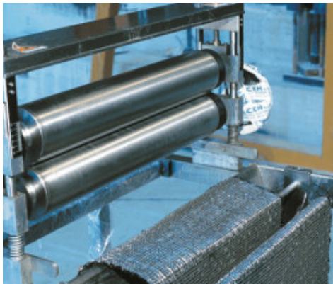
Impregnation of MapeWrap fabrics by machine
