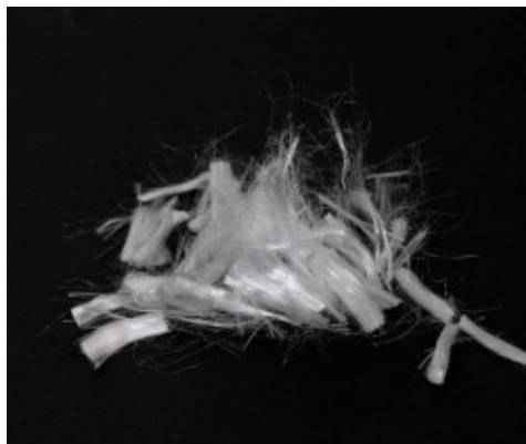
Mapefibre AT 06 FP monofilament microfibres
